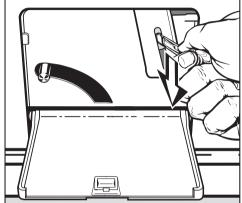
■ Insert a screwdriver into the notch, beside the lever, pull it down. The door will now open.
